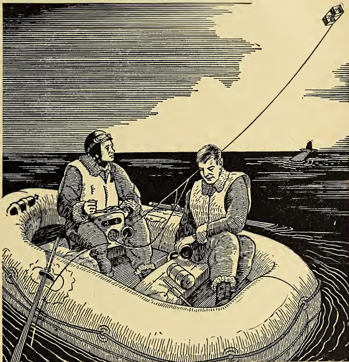
A portable radio device makes early rescue possible for survivors of forced landings at sea.
